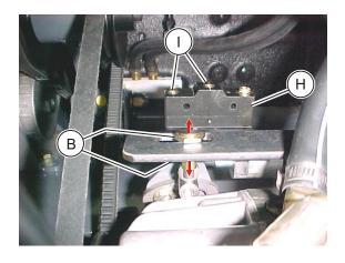
NOTE: Continuity tester leads at the middle and left terminals (I) will show continuity when the switch is "ON".
