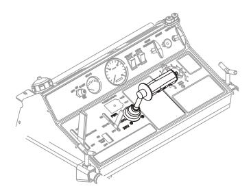
15. Position the Forward/Reverse Lever in the "Neutral" position. Following all safety and operational procedures, test that the engine cranks and starts.
