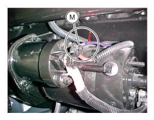
10. Remove nut holding existing purple wire on starter solenoid (M). Cut eyelet off of this wire (arrow).
