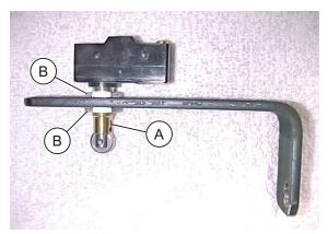
Fit switch plunger rod (A) through slot on bracket. Position about halfway and leave adjuster nuts (B) loose enough for later adjustment.
