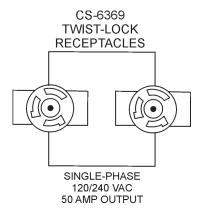
Figure 10. 120/240V Twist-Lock Auxiliary Receptacles
