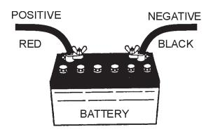
Figure 38. Battery Connections
