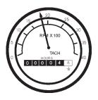
Figure 50. Engine Tachometer
