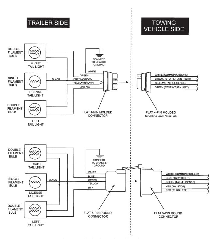
Figure 60. Trailer/Towing Vehicle Wiring Diagram
