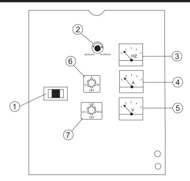
**Figure 6. Generator Control Panel**
