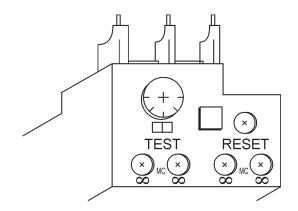
Figure 14. Over Current Relay
