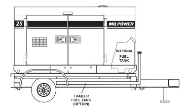
Figure 32. Internal Fuel Tank System
