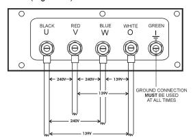
Figure 23. Output Terminal Lugs 3Ø-240/139 Three Phase Connections
