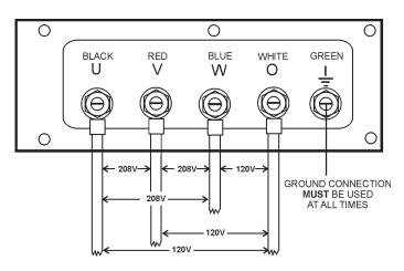
Figure 26. Output Terminal Lugs 3Ø-208/120V Connections
