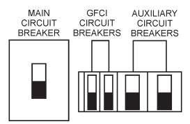
Figure 39. Main, Aux. and GFCI Circuit Breakers (OFF)
