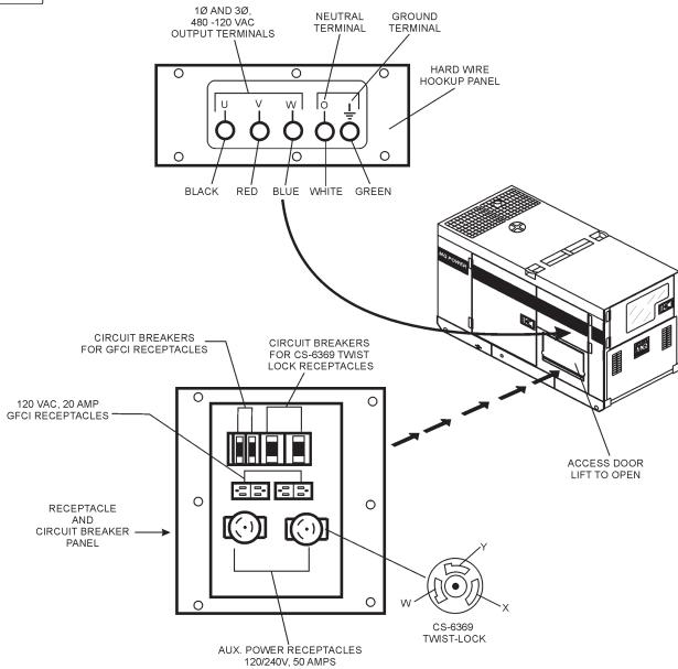
Figure 8. Output Terminal Panel
