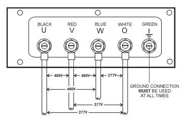
Figure 28. Output Terminal Lugs 3Ø-480/277V Three Phase Connections
