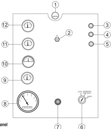
Figure 7. Engine Operating Panel
