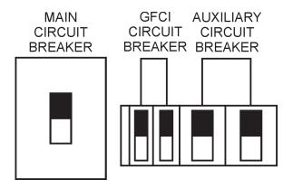
Figure 51. Main, AUX. and GFCI Circuit Breakers (ON)
