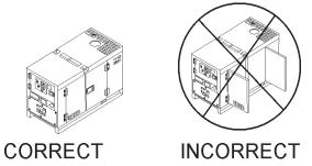
Figure 40. Engine Enclosure Doors
