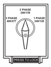
Figure 16. Voltage Selector Switch
