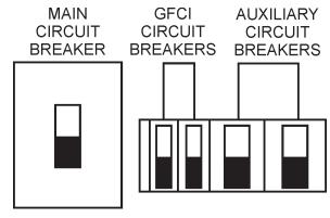
Figure 53. Main, AUX. and GFCI Circuit Breakers (OFF)
