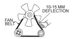
Figure 37. Fan Belt Tension
