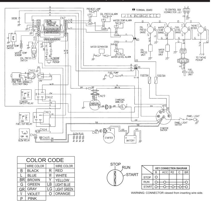
Figure 62. Engine Wiring Diagram
