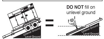
Figure 33. Only Fill on Level Ground
