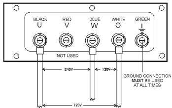
Figure 30. Output Terminal Lugs 1Ø-240/120V Connections
