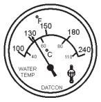
Figure 49. Coolant Temperature Gauge
