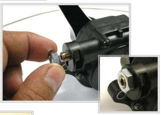
Insert throttle cable in the throttle cable sleeve. Pull sleeve up to housing and connect with earlier installed jam nut. Tighten outer jam nut to lock in place.
