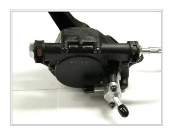
Loosen and remove the outer throttle adjuster jam nut.
