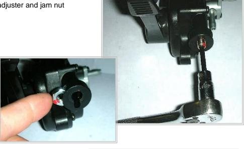
Behind the throttle adjuster is a slider. Pushing the inner cable from the opposite side of lever will push out the slider. Use a pick or small screwdriver to work the slider and throttle cable out of the housing.
