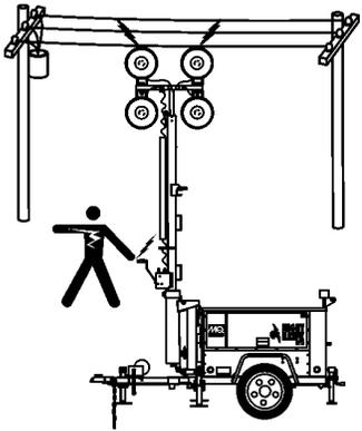
The lighting system of Stow's LT-12 Series Light Tower is comprised of 4 "Metal Halide" 1000 watt lamps. Each lamp has an output of 110,000 lumens yielding a total of 440,000 lumens for all four floodlights. Typical lighting coverage is between 5 to 7 acres.
