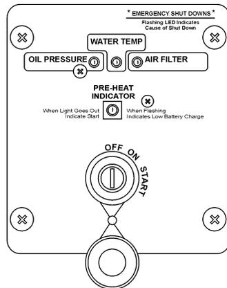
7. **Air Filter Indicator Alarm Light** – This alarm light flashes when a problem with the air filter is detected. Service as required.
