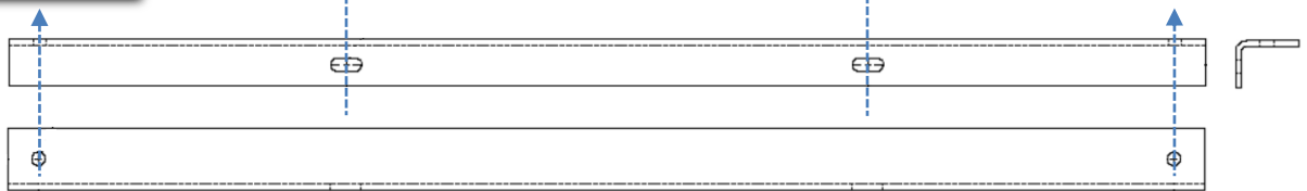
SUPPORT BRACKET – BOTTOM, FRONT FUEL TANK
