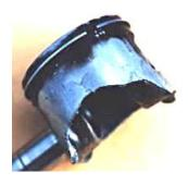
The skirt of this piston shattered because the piston cylinder clearance was too great. When the piston is allowed to rattle in the cylinder bore, it develops stress cracks and eventually shatters.
