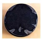
The crown of this piston shows an ideal carbon pattern. The transfer ports of this 2 stroke engine are flowing equally and the color of the carbon pattern is chocolate brown. That indicates that this engine's carb is jetted correctly.
