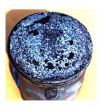
This piston crown has an ash color, which shows that the engine has run hot. The ash color is actually piston material that has started to flash (melt) and turned in to tiny flakes. If the engine was run any longer, it probably would've developed a hot spot and hole near the exhaust side and failed. The main causes of this problem are to lean carb jetting, too hot spark plug range, too far advanced ignition timing, too much compression for the fuels octane, or a general overheating problem.
