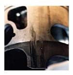
This piston was seized on the intake side. This is very uncommon and is caused by only one thing, loss of lubrication. There are three possible causes for loss of lubrication, no premix oil, separation of the fuel and pre-mix oil in the fuel tank, water passed through the air filter and washed the oil film off the piston skirt.
