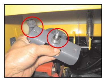
REPOSITION THE ASSEMBLY INTO THE CONSOLE SLOTS VIA THE UNDERSIDE OF THE CONSOLE AND MAINTENANCE ACCESS PANEL
