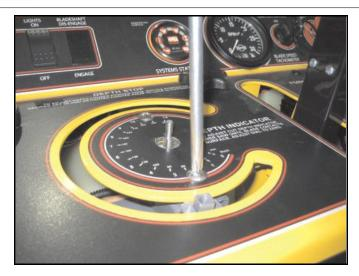
SECURE THE DEPTH STOP **ASSEMBLY TO THE CONSOLE** WITH (2) SCREWS (LOCTITE (BLUE) RECOMMENDED). **INSURE THAT SHAFT IS CENTERED AND THAT THERE** IS NO BINDING WITH THE **ROTATION OF THE DEPTH** STOP POINTER ARM.
