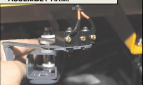
CORRECTLY REATTACH WIRING AND POSITION SWITCH ON THE DEPTH STOP POINTER ARM.
