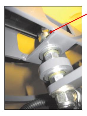
IF NECESSARY (VIA THE UNDERSIDE OF THE CONSOLE) REMOVE THE "OLD" DEPTH STOP ASSEMBLY BY RELEASING THE LOCK NUTS
