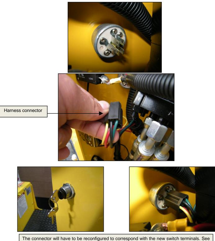
page one, terminal configuration is different between old switch and new switch.
