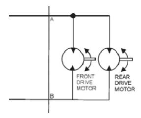
In order for you to test each motor individually you must eliminate the other motor.
