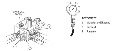
Disconnect hoses (I)(J) at the manifold block and plug the manifold block ports.
