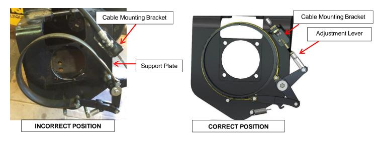
The bracket position is not visible but can be determined by feeling behind the support plate by hand.
