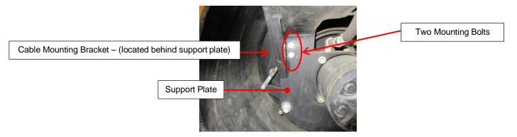
If bracket is discovered mounted upside down. The position can be corrected without removing main support plate.
