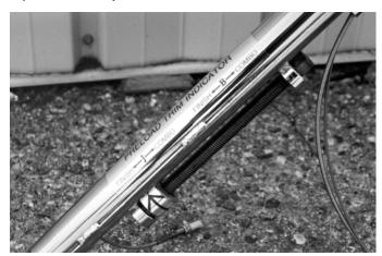
If you want to be able to increase the blade pitch using less arm force, adjust the block away from the gearbox. Be aware, this will also require more force to decrease the blade pitch. If you want to be able to decrease the blade pitch using less arm force, adjust the block toward the gearbox.
