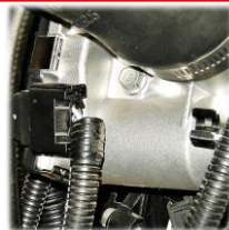
Throttle Position Sensor/Idle Speed Control Actuator. P/N 35100-2B140
