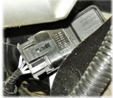
Manifold Absolute Pressure (MAP) Sensor P/N 39300-2B000
