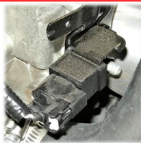
Radio Frequency (RF) noise cancelation unit for electrical system
