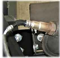
Oxygen Sensor, Pre Catalyst / Muffler P/N 201280
