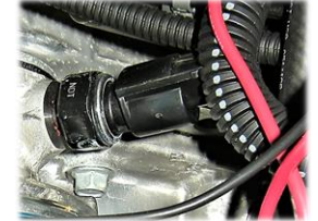
Oil Pressure Switch (NO) P/N 94750-37100
