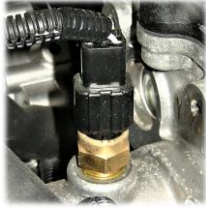
Coolant Temperature Sensor (230° F Shutdown) P/N 25600-2BF00
