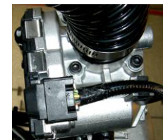
Throttle Position Sensor/Idle Speed Control Actuator (TPS/ISCA) Electronic throttle control incorporates the TPS in a feedback loop enabling the control.
