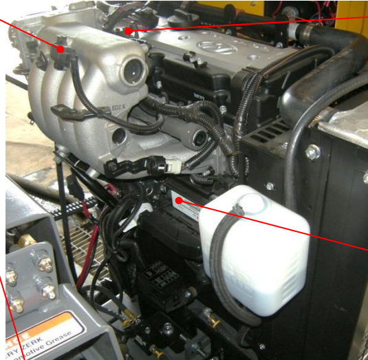
Manifold Absolute Pressure & Intake Air Temperature Sensor (MAP & IAT Sensor) Provides instant manifold pressure & temp information to the engine's ECU.
