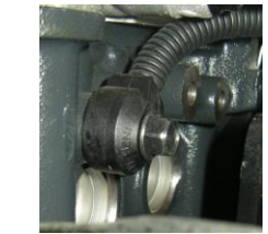
(Knock Sensor) Senses engine vibrations caused by engine knock, ECU will adjust timing to compensate if needed.
