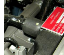
Positive Crankcase Ventilation Valve (PCV Valve) Only one part of the PCV system whereby crankcase gases return to the air intake.
