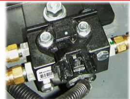
(Gasoline Fuel Rail Sensor) ECU monitors Temperature & Pressure via this sensor.
