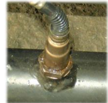
Oxygen Sensor 2/post-cat (HO2S Sensor 2) specifically used for controlling the air to fuel ratio of the engine.
