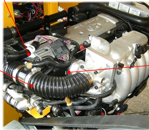
Engine Control Unit (ECU) Controls actuators via data from a series of sensors ensuring optimal eng. performance.
