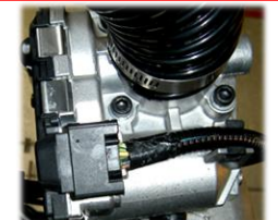
Engine Control Unit (ECU) Controls actuators via data from a series of sensors ensuring optimal eng. performance.
