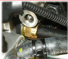
Coolant Temperature Sensor The ECU adjusts various eng systems based on variabe coolant temperature data.
