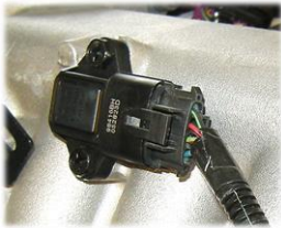
Manifold Absolute Pressure & Intake Air Temperature Sensor (MAP & IAT Sensor) Provides instant manifold pressure & temp information to the engine's ECU.
