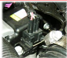
Top Dead Center/CAM Position Sensor (TDC/CMPS) CAM & CRANK positions data to ECU together derive the current combustion cycle.
