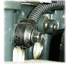
(Knock Sensor) Senses engine vibrations caused by engine knock, ECU will adjust timing to compensate if needed.
