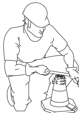
Figure 41-D. Slump Test (Removing Excess Concrete)
