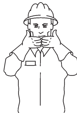
ALL DONE CLEAN-UP
