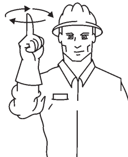
START PUMP SPEED UP
