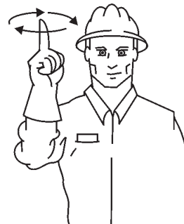
START PUMP SPEED UP
