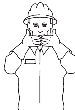
ALL DONE CLEAN-UP
