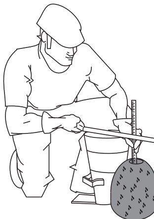
Figure 38-F. Slump Test (Measurement)
