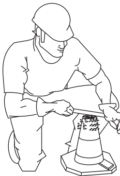
Figure 38-D. Slump Test (Removing Excess Concrete)
