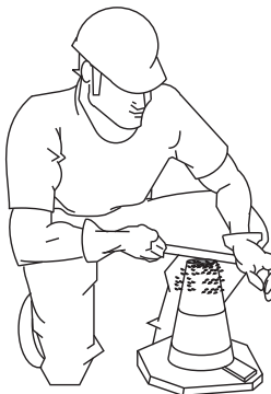
Figure 34-D. Slump Test (Removing Excess Concrete)
