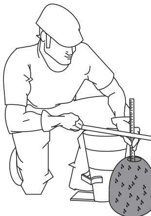
Figure 34-E. Slump Test (Cone Invert)
