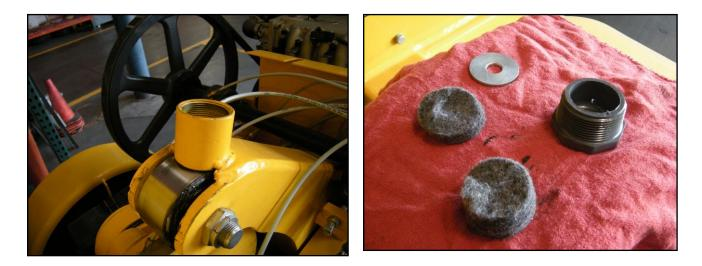
The cam rocker arm felt pads are part of maintenance and should be checked regularly.
