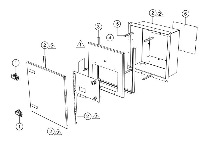
NOTES 1 Modified Cummins Power Command Digital Generator Set Control 2 All items # 2 are part of EE56469 Assembly.
