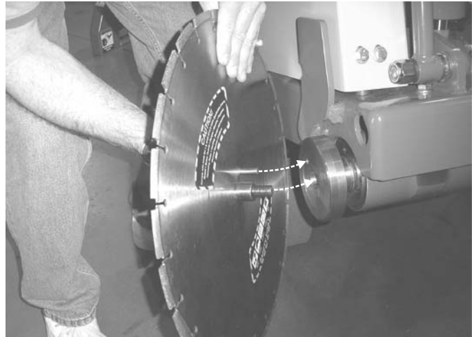
Figure 11. Aligning Flange Pin Through Blade (Standard Blade Flange System shown)
