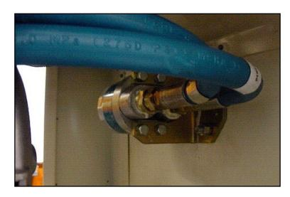
**13.** Oil level may drop due to the additional hoses, replace oil as needed.
