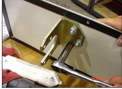
**6.** Mount the bracket to the panel with mounting hardware.
