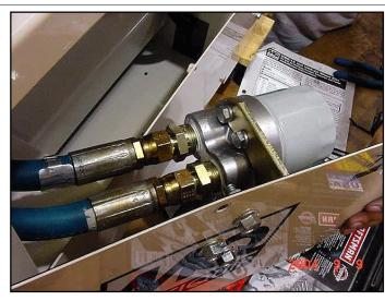
**11.** Use tie straps to hold hoses in place. Make sure the hoses are high enough to cause the oil to flow back down into the engine.
