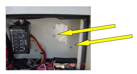
**RE1 & R** is mounted behind the panel by machined screws
