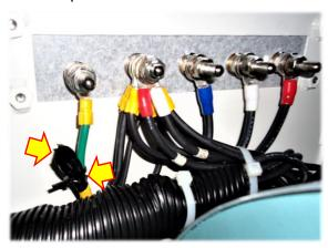
5) Install green ground wire, flat and lock washers plus the nut to the ground lug stud. Ref. below torque table for nut.
