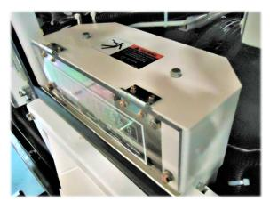
8) WARNING: After removing the neutral bond the MQ Warning Decal (part #EE58626) must be placed on or near the output panel door
