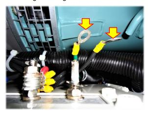
6) Insulate the ring terminal of the black neutral bond jumper wire so that no bare metal is exposed. Secure it to the green ground wire with a small tie wrap
