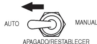
Figura 54. interruptor de control MPEC (AUTO)
