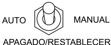
**Figura 55. Interruptor de control MPEC (Off/Reset)(Apagado/Restablecer)**
