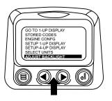
Once the "Adjust Backlight" menu item has been highlighted touch the "Enter Button" to activate the "Adjust Backlight" function
