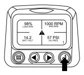
Touching the "Enter Button" once again will hide the fault and return the screen to the single or four parameter display.0
