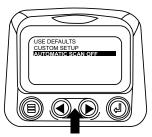
16. Touching the "Enter Button" toggles the "Automatic Scan" function on.
