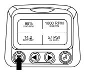
2. The main menu will pop up on the display. Use the "Arrow Buttons" to scroll through the menu until "Adjust Contrast" is highlighted.
