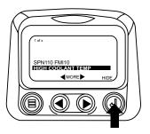
The display will return to the single or four parameter display but the display will contain the "Active Fault" warning icon. Touching the "Enter Button" will redisplay the hidden fault.
