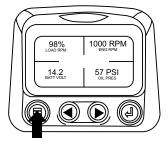
2. The main menu will pop up on the display. Use the arrow buttons to scroll through the menu until the "Select Units" is highlighted.
