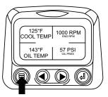
2. The main menu will be displayed. Use the "Arrow Buttons" to scroll through the menu until the "Utilities" is highlighted.
