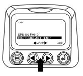
5. Touch the "Menu Button" to exit the Main menu and return to the engine parameter display.
