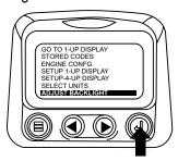
4. Use the "Arrow Buttons" to select the desired backlight intensity..
