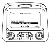
3. To acknowledge and "Hide" the fault and return to the single or four parameter display touch the "Enter Button"
