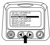
3. Once the "Engine Configuration" menu item has been highlighted touch the "Enter Button" to view the engine configuration data.
