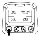
When the PowerView receives a fault code from an engine control unit the single or four parameter screen will be replaced with the "Active Fault Codes" message.
