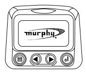
The "Wait to Start" message will be displayed for engines with a pre-startup sequence. Once the "Wait to Start" message is no longer displayed the operator may start the engine. Note: Displays only when SAE J1939 message is supported by engine manufacturg.
