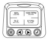
2. The main menu will pop up on the display. Use the "Arrow Buttons" to scroll through the menu until the Stored Fault Codes is highlighted.
