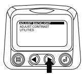
4. Touch the Arrows" to scroll to the desired menu item or touch "Menu" to exit the Main menu and return to the engine parameter display.
