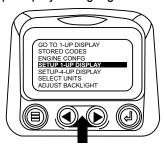
3. Once the "Setup 1-up Display" menu icon has been highlighted touch the "Enter Button" to access the "Setup 1-up display" function.
