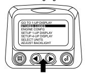
Once the "Stored Fault Codes" menu item has been highlighted touch the "Enter Button" to view the "Stored Fault Codes" (when applicable, consult engine or transmission manufacturer for SAE J1939 supported parameters
