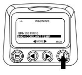
The Single or Four parameter screen will display the fault icon until the fault condition is corrected. NOTE: Ignoring active fault codes could result in severe engine damage.
