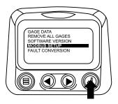
4. Use the "Arrows" to scroll down to and highlight either the "Slave Active or Master Active" modes. Touch the "Enter" button to toggle between master and slave.
