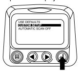
9. Touching the "Enter Button" will display a list of engine parameters.
