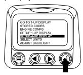
Touch the "Enter Button" to activate the "Use Defaults" function. This action will reset the unit to the factory default.
