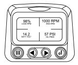
2. The main menu will pop up on the display. Use the "Arrow Buttons" to scroll through the menu until the Stored Fault Codes is highlighted.
