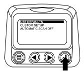
The "Use Defaults" screen will be displayed during the resetting period then will automatically return to the "Setup 4- Up Display" menu.
