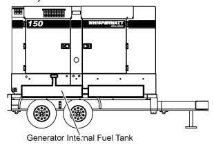
Figure 30. Internal Fuel Tank System
