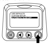
18. Once the "Use Defaults", "Custom Setup" and "Automatic Scan" functions have been set touch the "Menu Button" to return to the main menu.
