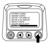
3. Once in the "Utilities" menu use the "Arrows" to scroll through the menu until the "Modbus Setup" menu is highlighted, then touch "Enter".
