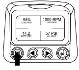
The main menu will pop up on the display. Use the "Arrow Buttons" to scroll through the menu until the "Setup 4-Up Display" is highlighted.
