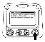
12. Use the "Arrow Button" to scroll and highlight the desired parameter that has not been selected for display.
