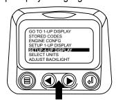
3. Once the "Setup 4-Up Display" menu item has been highlighted touch the "Enter Button" to activate the "Setup 4- Up Display" menu.
