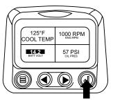
The parameter that is highlighted is the selected parameter for the screen. Use the "Arrow Buttons" to highlight the new parameter to be placed in the quadrant selected in the previous screen.
