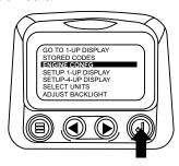
4. Use the "Arrow Buttons" to scroll through the engine configuration data.
