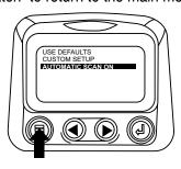
19. Touch the "Menu Button" to exit the Main menu and return to the engine parameter display.
