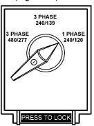
Figure 39. Voltage Selector Switch STARTING (MANUAL)
