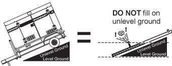
Figure 19. Only Fill on Level Ground
