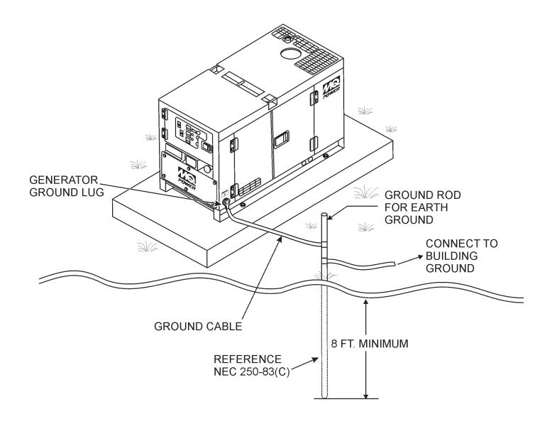
**Figure 2. Typical Generator Grounding Application**
