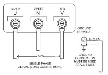
Figure 16. Output Terminal Lugs 240 VAC Single Phase Connections
