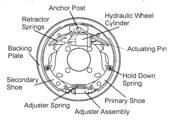
Figure 37. Hydraulic Brake Components
