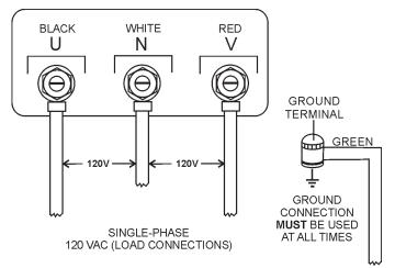
Figure 12. Output Terminal Lugs 120 VAC Single Phase Connections
