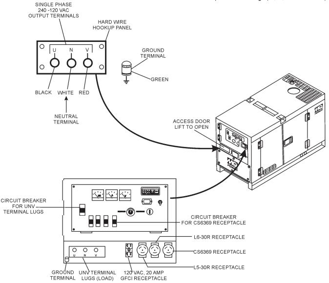
**Figure 5. Output Terminal Panel**
