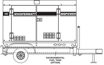
Figure 18. Internal Fuel Tank System
