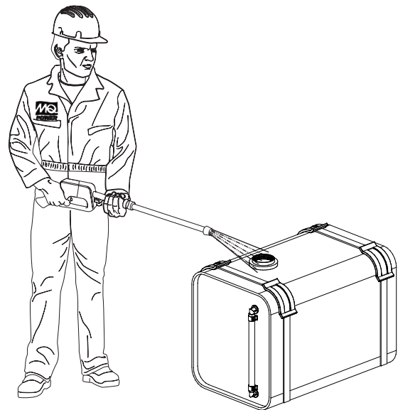
Figure 44. Cleaning The Fuel Tank
