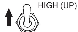
**Figure 28. Engine Speed Switch (High)**
