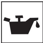
If this lamp is ever lit (**ON**) during normal operation of the generator, the emergency shutdown system will stop the engine automatically.
