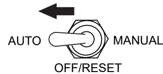
Figure 61. Auto Start/Stop Switch (Auto Position)
