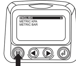
7. Touch the “Menu Button” to exit the Main menu and return to the engine parameter display.
