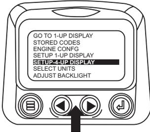
3. Once the “Setup 4-Up Display” menu item has been highlighted touch the “Enter Button” to activate the “Setup 4-Up Display” menu.
