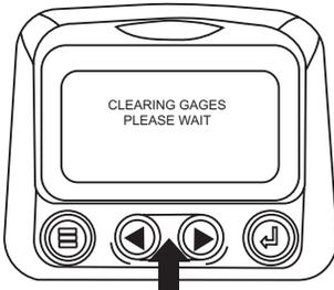
8. When the gage data has cleared, the display automatically returns to the “Utilities” menu. Scroll to “Software Version”. Touch “Select” to view the software version currently in the diagnostic display.
