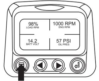
2. The main menu will pop up on the display. Use the “Arrow Buttons” to scroll through the menu until the “Setup 1-up Display” is highlighted.
