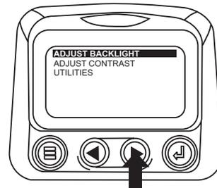
4. Touch the “Arrows” to scroll to the desired menu item or touch “Menu” to exit the Main menu and return to the engine parameter display.
