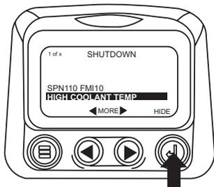
4. The display will return to the single or four parameter display, but the display will contain the "Shut Down" icon. Touching the "Enter Button" will redisplay the hidden fault.
