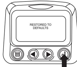
8. Custom Setup- To perform a custom setup of the 1-Up Display, use the arrow buttons to scroll to and highlight “Custom Setup” on the display.
