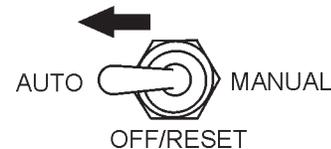
**Figure 55. MPEC Control Switch (AUTO)**
