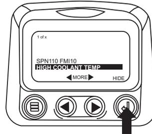
5. The display will return to the single or four parameter display but the display will contain the “Active Fault” warning icon. Touching the “Enter Button” will redisplay the hidden fault.
