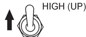
Figure 43. Engine Speed Switch (High)
