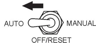
Figure 55. MPEC Control Switch (AUTO)
