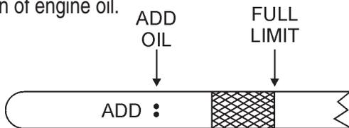
Figure 30. Engine Oil Dipstick
