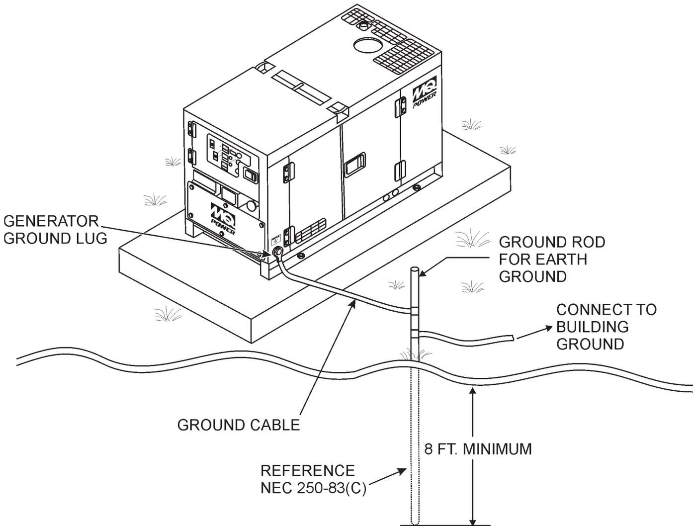
Figure 4. Typical Generator Grounding Application
