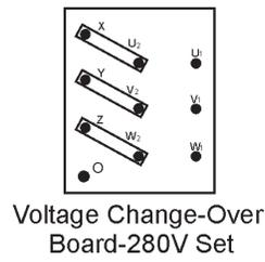
Figure 63. Generator Wiring Diagram
