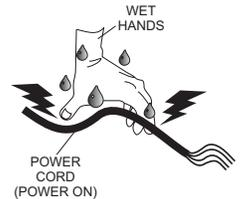
**NEVER** touch output terminals during operation. This is extremely dangerous. **ALWAYS** stop the machine and place the circuit breaker in the **OFF** position when contact with the output terminals is required.
