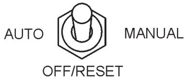
**Figure 57. MPEC Control Switch (Off/Reset)**
