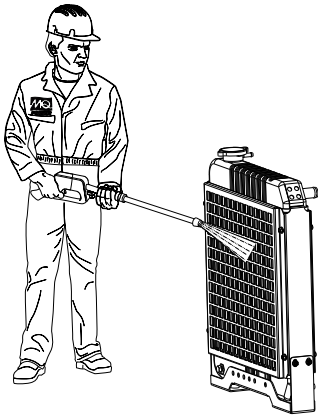
Figure 71. Cleaning The Radiator
