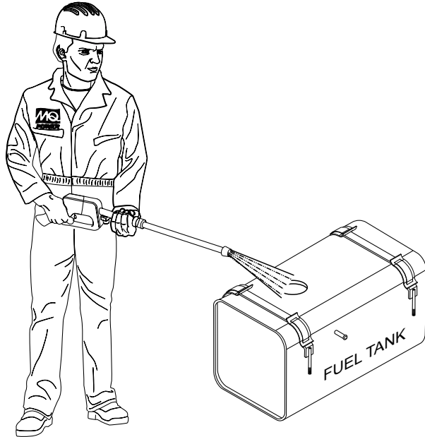
Figure 66. Cleaning The Fuel Tank
