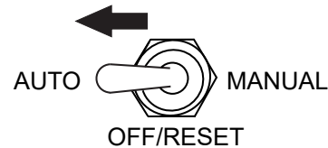
Figure 57. Auto Start/Stop Switch (Auto Position)
