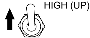
Figure 56. Engine Speed Switch (High Position)
