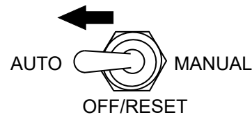
Figure 57. Auto Start/Stop Switch (Auto Position)
