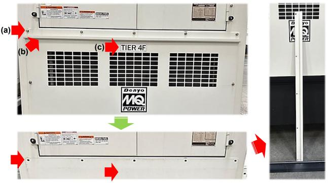
NOTE: Existing Bolts are Too Short to Mount the Grab Handle. Replace with: M8x25 Bolts, Washers, Lock Washers
