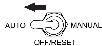
Figure 64. Auto Start/Stop Switch (Auto Position)
