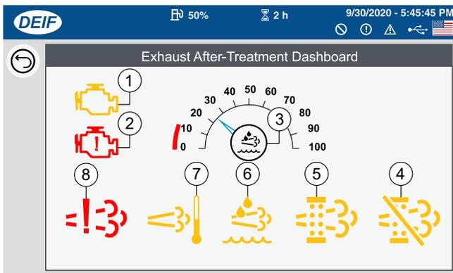
**Figure 194. Exhaust After-Treatment Dashboard Indicators**
