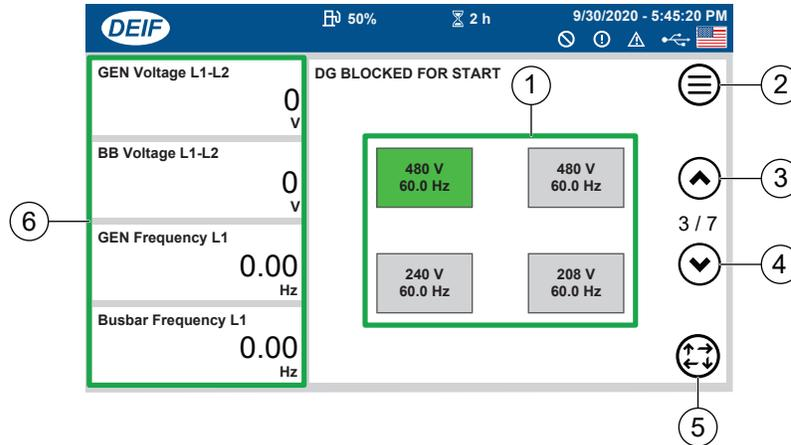
Figure 213. Voltage Selection Screen (3 of 7)
