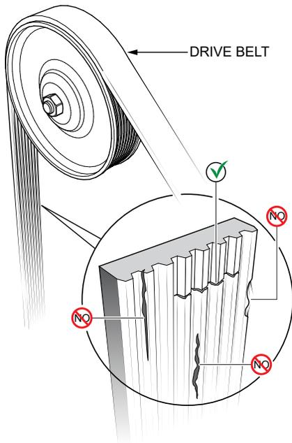
**Figure 186. Drive Belt Inspection**
