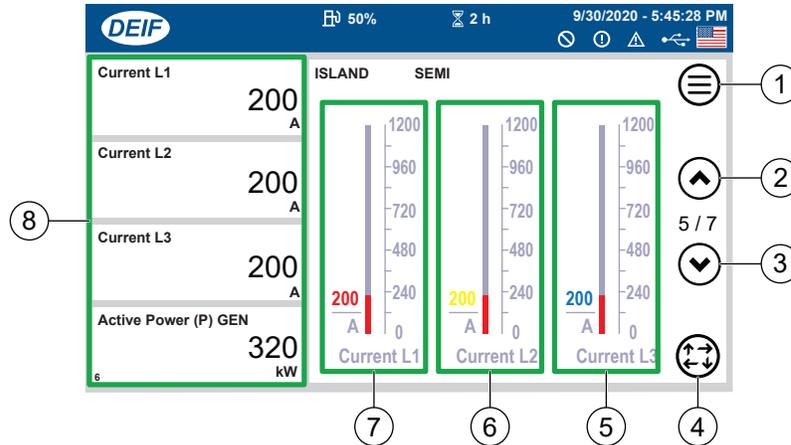
Figure 215. Generator Amperage Screen (5 of 7)
