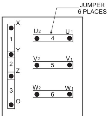
**Figure 14. Voltage Change-Over Board
