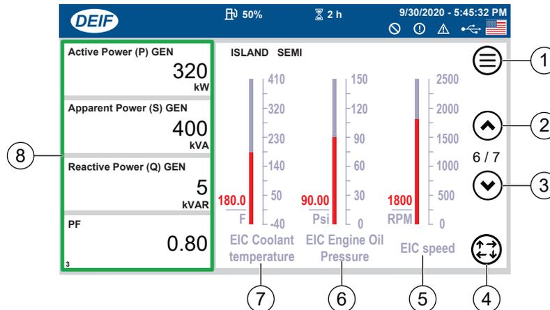
Figure 216. Engine Data Screen (6 of 7)
