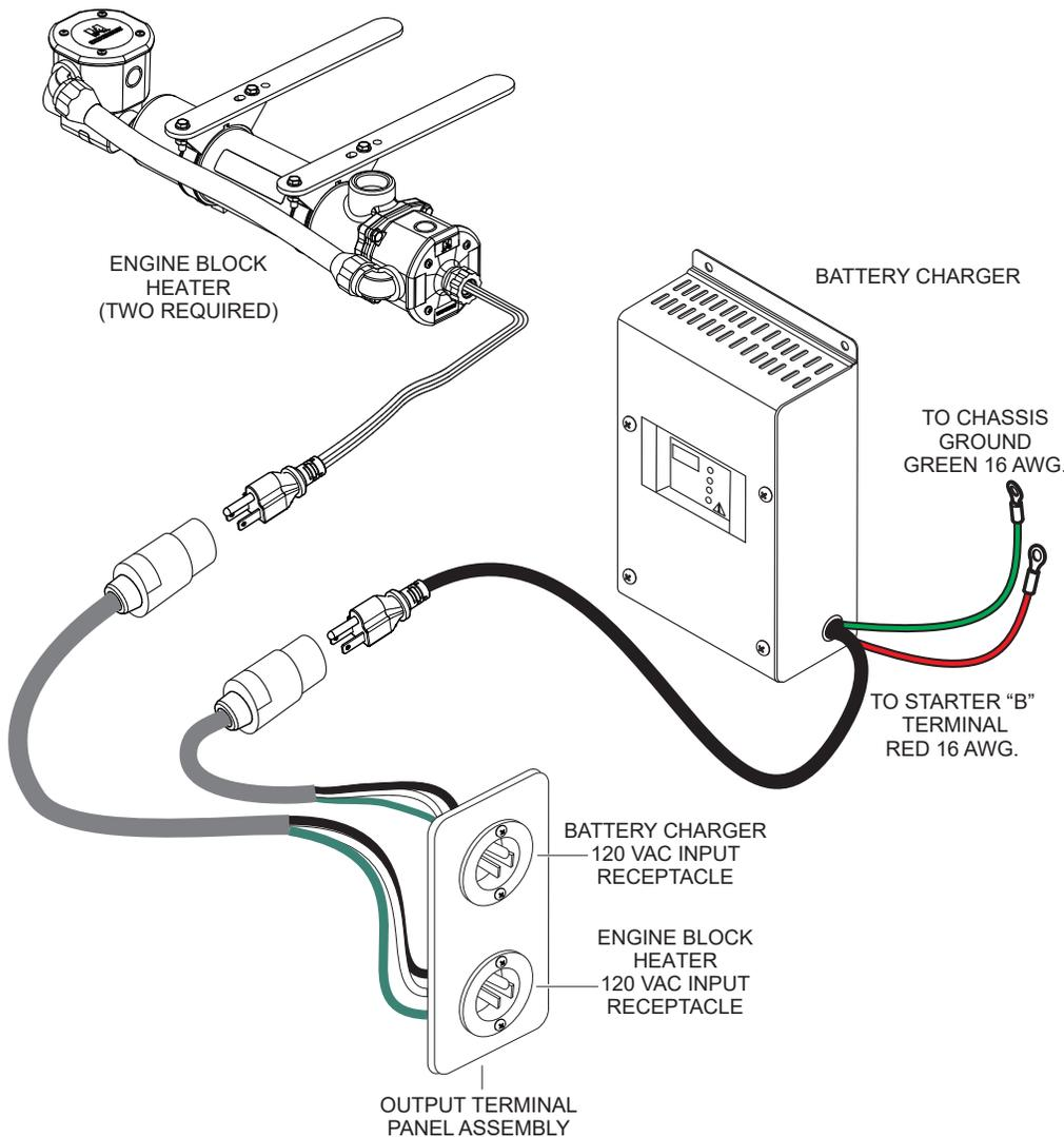
Figure 192. Engine Block Heater And Battery Charger
