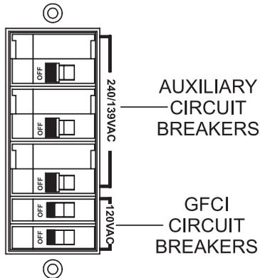
**Figure 74. GFCI and Auxiliary Circuit Breakers (OFF)**
