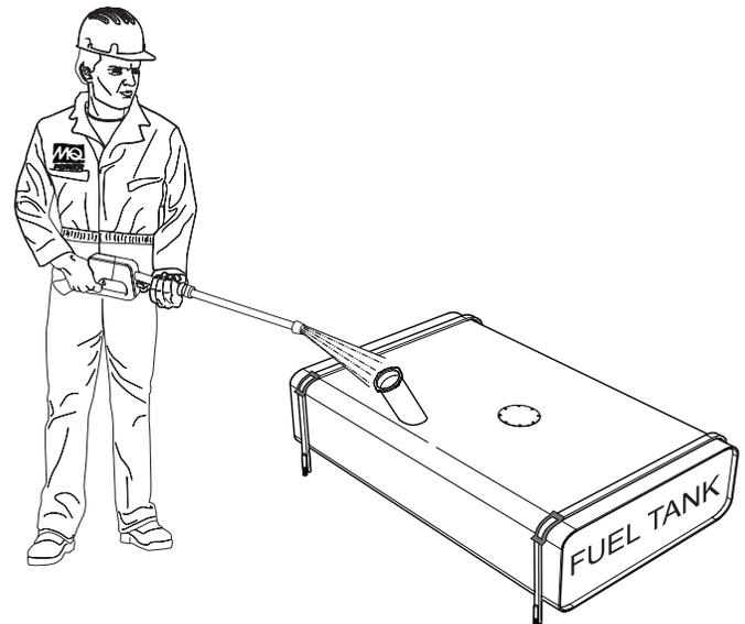
**Figure 180. Cleaning The Fuel Tank**
