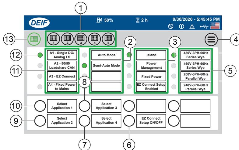
**Figure 224. Main Additional Operator Panel (AOP) Screen**
