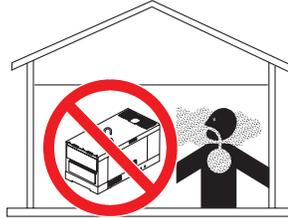
■ When operating the generator outdoors, **DO NOT** place the generator near doors, windows or vents that could allow carbon monoxide to enter and build up in occupied spaces.
