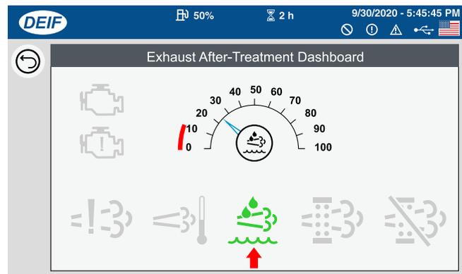
**Figure 199. Exhaust After-Treatment Dashboard (Check DEF Indicator)**
