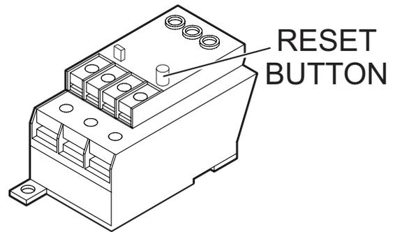
Figure 11. Overcurrent Relay
