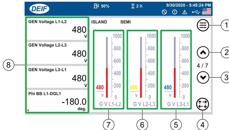
Figure 214. Output Voltage Status Screen (4 of 7)
