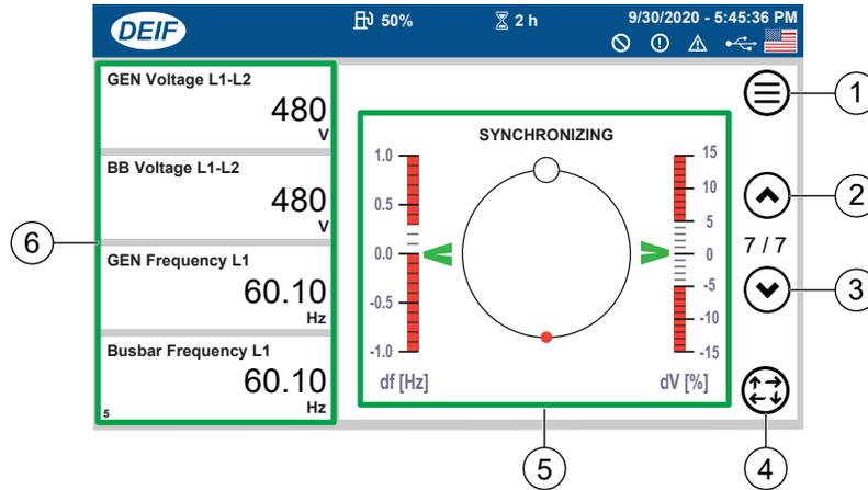
Figure 217. Synchronization Status Screen (7 of 7)
