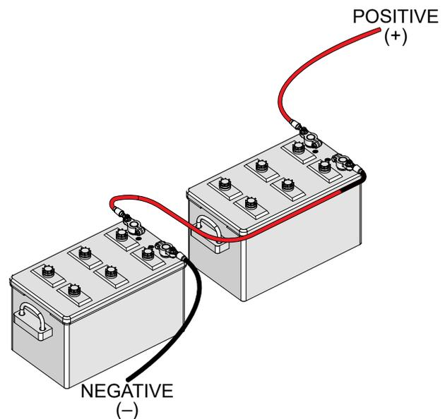
Figure 34. Battery Connections
