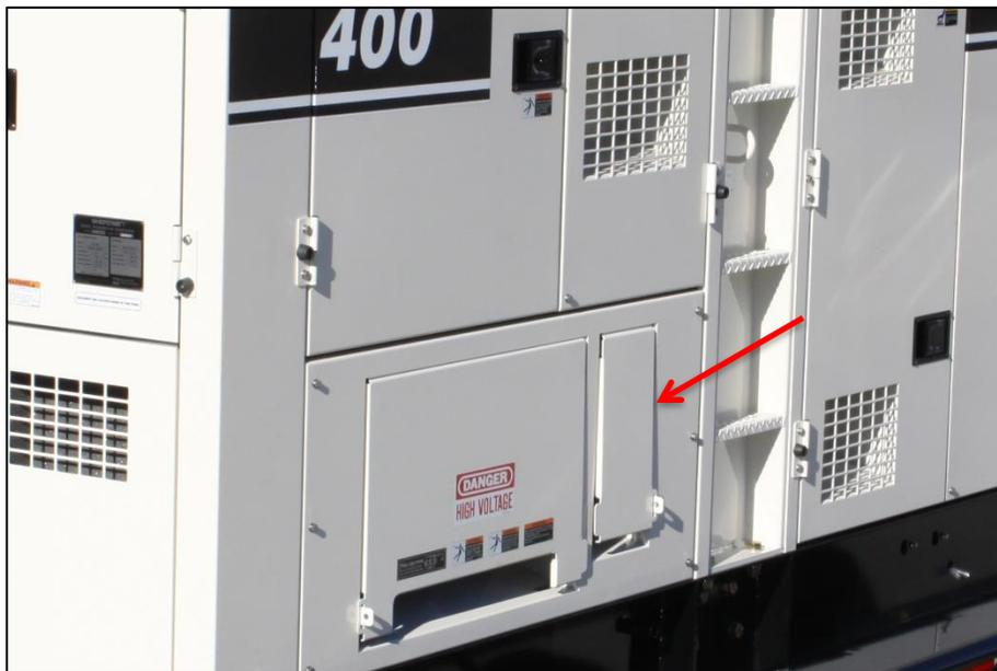
2. Remove the 6 bolts holding this panel to the side of the unit. Once the retaining hardware has been removed, tilt the panel forward to access the back.
