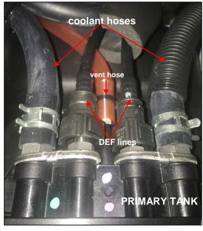
From the left DEF tank, inspect the vent port and check if a red vacuum cap is present. The cap should be removed and a new vent hose must be installed immediately.
