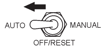
Figure 54. MPEC Control Switch (AUTO)
