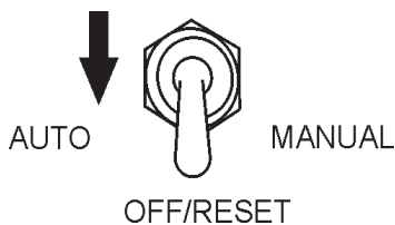
Figure 56. MPEC Control Switch (Off/Reset)
