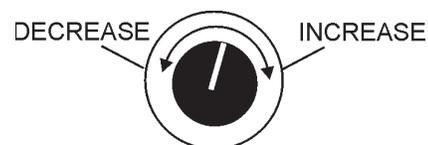
Figure 26. Voltage Regulator Knob (208V)
