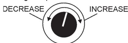
Figure 23. Voltage Regulator Knob (139V/240V)
