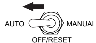
Figure 58. Auto Start/Stop Switch (AUTO)
