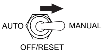
Figure 46. Auto Start/Stop Switch (Manual Position)
