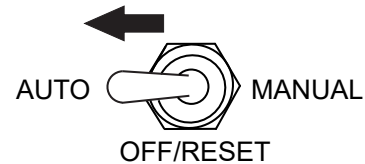
Figure 58. Auto Start/Stop Switch (Auto Position)
