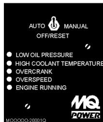
If the engine does not engage (start) by the third attempt, the engine will be shutdown by the engine controller's Over Crank Protection mode. If the engine engages at a speed (RPM's) that is not safe, the controller will shutdown the engine by initializing the Over Speed Protection mode.
