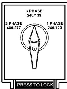
Figure 14. Voltage Selector Switch
