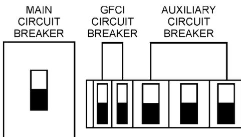
**Figure 56. Main, GFCI and Load Circuit Breakers (OFF)**
