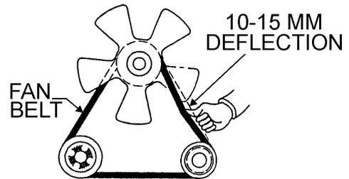
Figure 37. Fan Belt Tension
