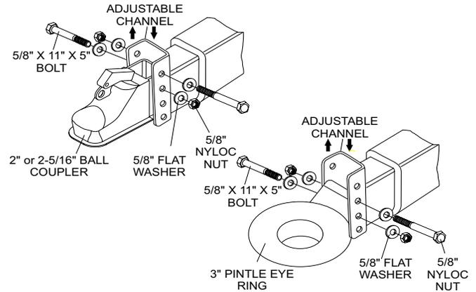
Figure 65. Adjustable Channel
