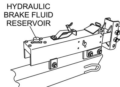
**Figure 64. Hydraulic Brake Actuator**
