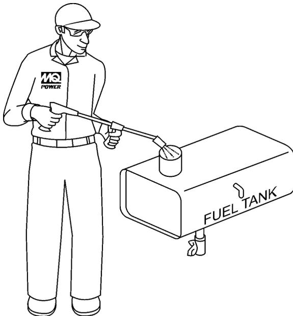
Figure 60. Fuel Tank Cleaning
