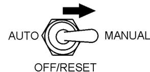
**Figure 43. MPEC Control Switch (Manual Position)**
