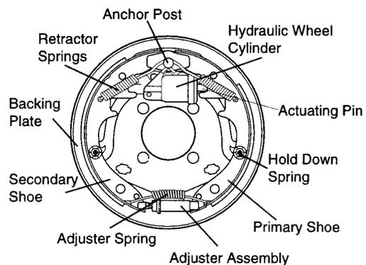
**Figure 63. Hydraulic Brake Components**
