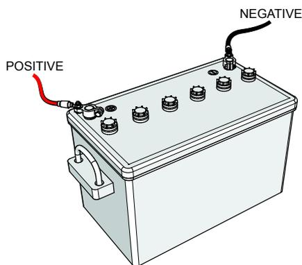
Figure 38. Battery Connections
