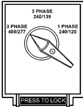
**Figure 28. Voltage Selector Switch
