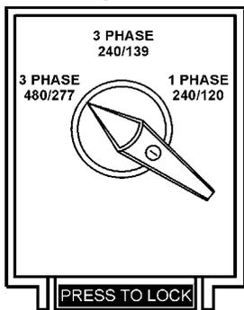
**Figure 24. Voltage Selector Switch
