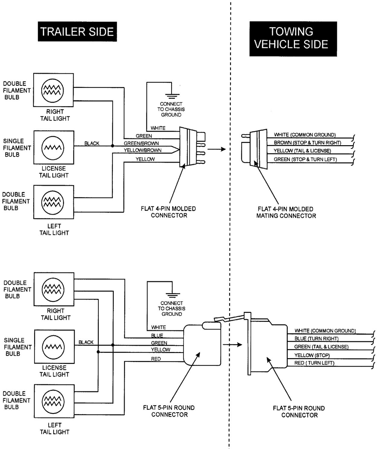
Figure 69. Trailer/Towing Vehicle Wiring Diagram
