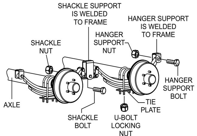
**Figure 67. Leaf Suspension Components**
