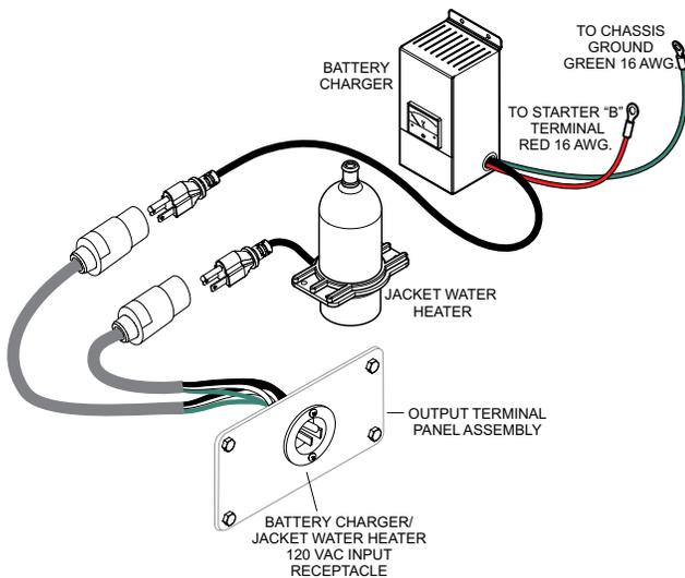
**Figure 62. Battery Charger and Water Heater Power Connections**
