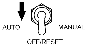
Figure 64. MPEC Control Switch (Off/Reset)
