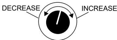
Figure 19. Voltage Regulator Knob
