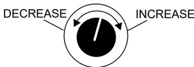
Figure 19. Voltage Regulator Knob
