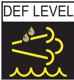
Figure 103. DEF Level Symbol
