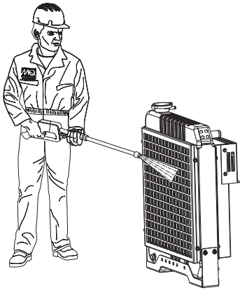
Figure 131. Cleaning The Radiator
