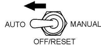
Figure 53. Auto Off/Reset Manual Switch (AUTO)
